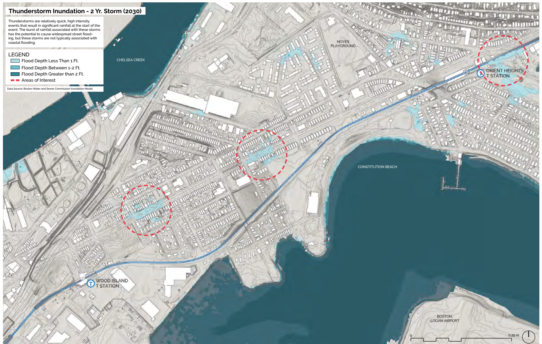
Thunderstorm Inundation - 2 Year Storm (2030) map created by Weston & Sampson (data source: Boston Water and Sewer Commission Inundation Model)
